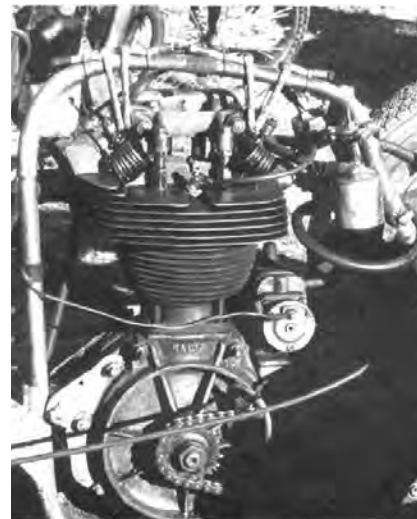
Above ES2 engine with stiffened drive-side crankcase. Below, early testing somewhere outside Sydney. Photos Graham Howard Collection.
